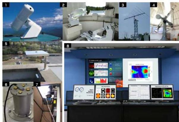
**Fig. 1 Observation systems in KASI. (1) Solar Flare Telescope, (2) Solar Imaging Spectrograph, (3)E-Callisto, (4) Sunspot Telescope, (5) Scintimon, (6) Magnetometer, (7) All Sky Camera, (8) Space weather monitoring Lab.**
