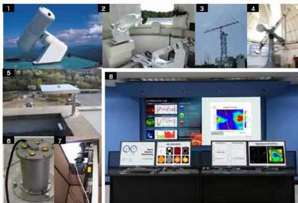
**Fig. 1** Observation systems in KASI. (1) Solar Flare Telescope, (2) Solar Imaging Spectrograph, (3)E-CALLISTO, (4) Sunspot Telescope, (5) SCINTMON, (6) Magnetometer, (7) All Sky Camera, (8) Space Weather Monitoring Lab.
